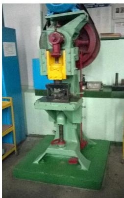
Fig. 1. Crank-press K116G, with 0.125 MN force
