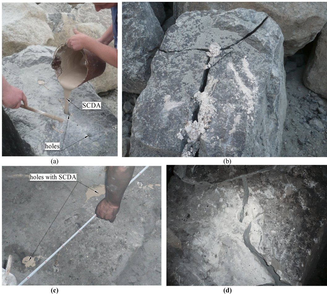
Fig. 14. Experiments in-situ: (a) pouring SCDA mixture into boreholes in granite; (b) fracturing of granite by conventional SCDA method; (c) pouring SCDA mixture into boreholes in sandstone; (d) fracturing of sandstone by conventional SCDA method.
