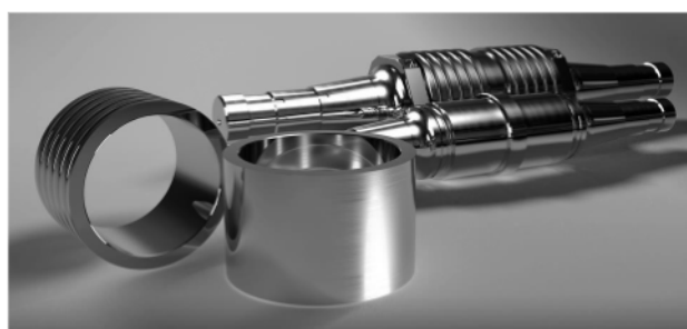
Fig. 2. Roller of small-grade rolling mill for rolling of a reinforcing profile with hard-alloy bandages (a bandage ring in a state of delivery, a bandage ring with the cut grooves, a steel axis of a roll, the bandaged roll assembled)
