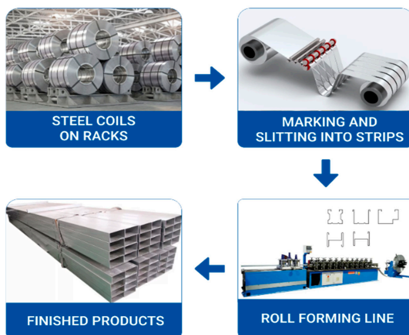
Figure 4. Organization of cold-formed steel sections production from galvanized coil steel.
