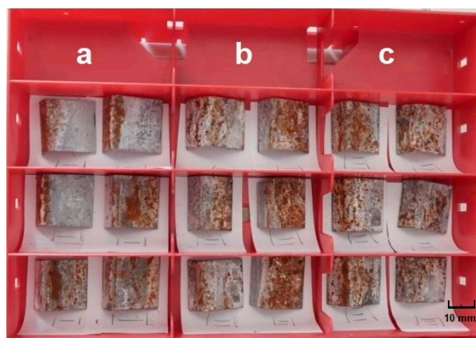
Figure 8. Test specimens cut from cold-formed hollow sections for chemical testing: (a) CFS (IV)— 30 \times 50 mm, t = 1.48 – 1.5 mm; (b) CFS (V)— 30 \times 50 mm, t = 1.5 mm; (c) CFS (VI)— 35 \times 49.5 mm, t = 1.5 mm.
